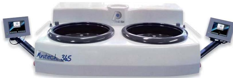
Width: 1036mm - Depth: 742mm - Height: 298mm
